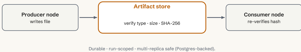
FIGURE 3 Effect-verified artifact hand-off between workflow nodes
